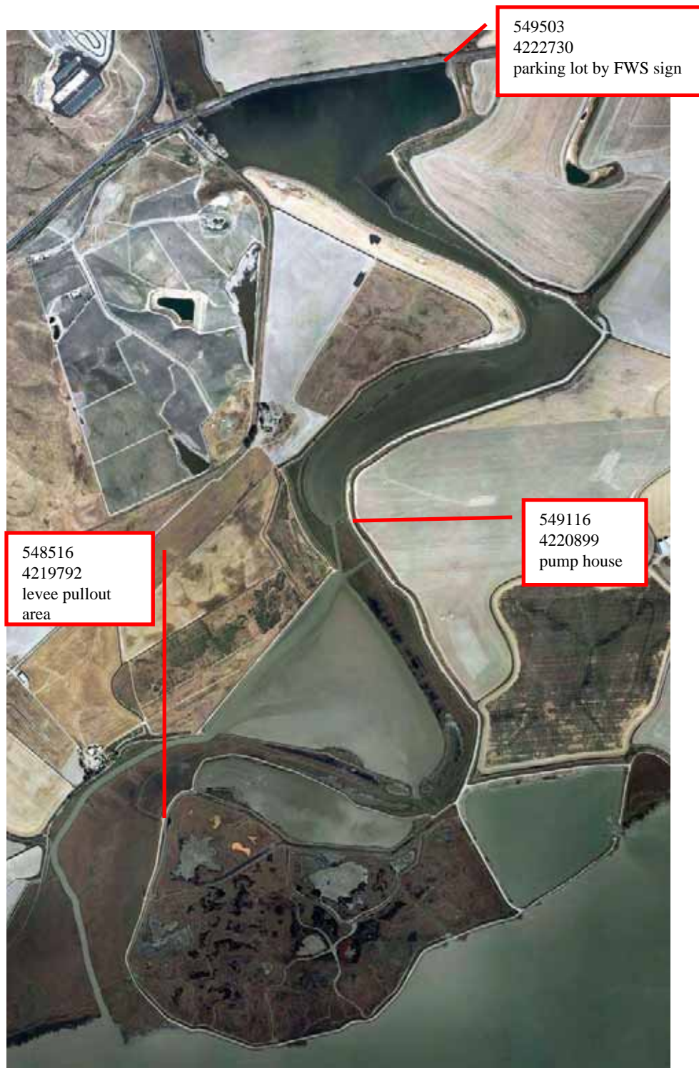
Figure 3. Location of benchmarks at Tolay Creek. Benchmarks were resurveyed in May 2003 by Shoreline Engineering. All GPS coordinates are recorded in NAD27 Zone 10 North. Several more benchmarks will be added and surveyed in 2005.
